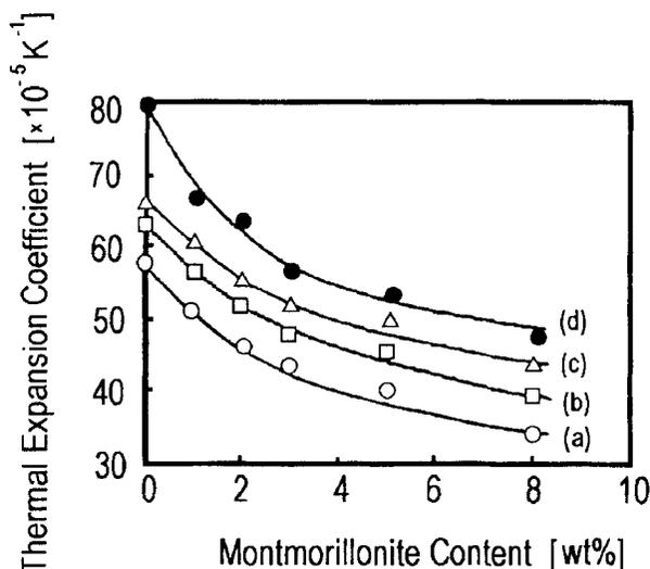
FIGURE 7 Montmorillonite content dependence of thermal expansion coefficient of polyimide-clay hybrid at: (a) 150°C, (b) 200°C, (c) 250°C, and (d) 250°C.
