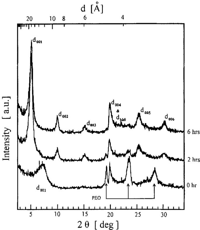
FIGURE 8 X-ray diffraction pattern of PEO/Na<sup>+</sup>-montmorillonite hybrid heated to 80°C for 0, 2 and 6 hours.
