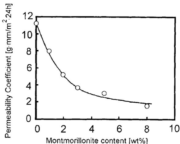
FIGURE 4 Montmorillonite content dependence of water vapor in polyimide-clay hybrid.
