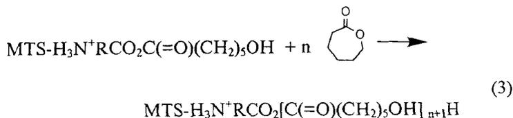
It is important to point out that the resulting PCL chains are ionically bound to the dispersed mica-type silicate (MTS) layers through the protonated amine terminus of the polymer, which restricts chain mobility.
