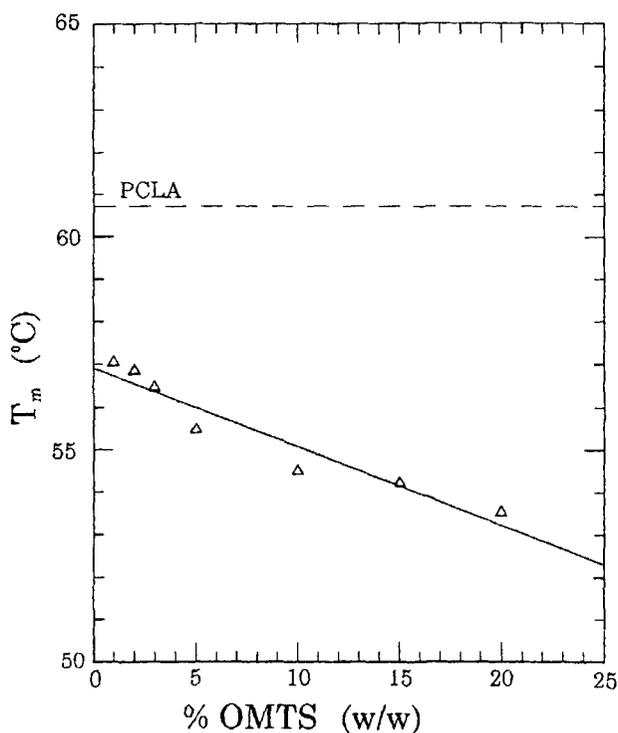
FIGURE 2 Plot of the temperature of onset of polymer melting *versus* weight fraction of OMTS in the PCLC nanocomposites. Dashed line corresponds to the melting temperature of PCLA.
