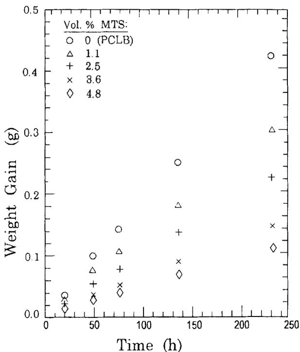
FIGURE 3 H<sub>2</sub>O weight gain of nanocomposite film-covered dessicators *versus* exposure time in a 75% relative humidity atmosphere. Data for nanocomposite films containing .011, .025, .036, and .048 volume fraction silicate are shown.
