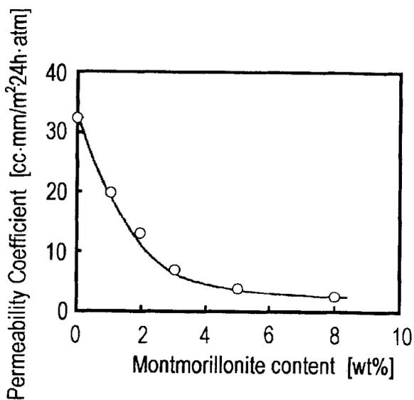
FIGURE 5 Montmorillonite content dependence of permeability coefficient of  $O_2$  in polyimide-clay hybrid.
