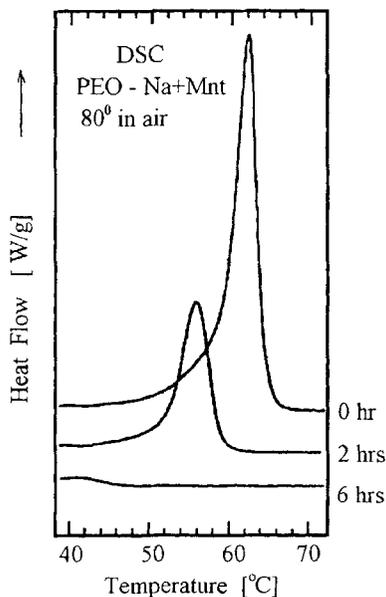
FIGURE 9 DSC traces for PEO/Na<sup>+</sup> - montmorillonite hybrids heated to 80°C for 0, 2 and 6 hours.
