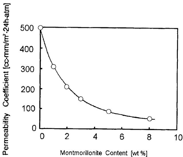
FIGURE 6 Montmorillonite content dependence of permeability coefficient of He in polyimide-clay hybrid.
