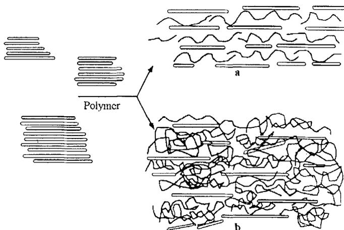
FIGURE 1 Schematic of composite structures obtained using layered silicates. The rectangular bars represent the silicate layers. (a) Single polymer layers intercalated in the silicate galleries (*intercalated hybrids*). (b) Composites obtained by delamination of the silicate particles and dispersion in a continuous polymer matrix (*delaminated hybrids*).
